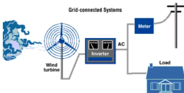
A 1.5-kilowatt (kW) wind turbine will meet the needs of a home requiring 300 kilowatt-hours (kWh) per month, for a location with a 6.26-meters-per-second (14-mile-per-hour) annual average wind speed. Most turbines have automatic speed-governing systems to keep the rotor from spinning out of control in very high winds. This information, along with your local wind speed distribution and your energy budget, is sufficient to allow you to specify turbine size.
