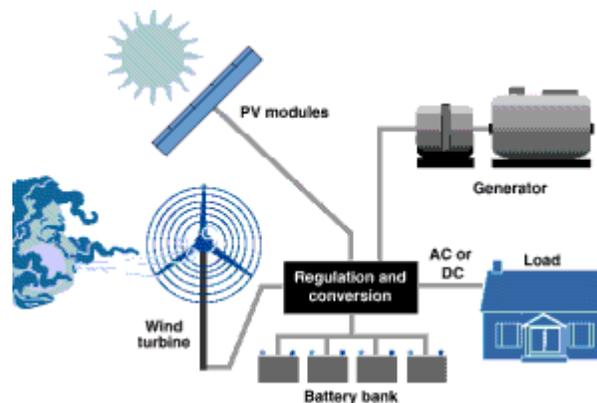
If the batteries run low, the engine-generator can be run at full power until the batteries are charged. Adding a fossil-fuel-powered generator makes the system more complex, but modern electronic controllers can operate these complex systems
