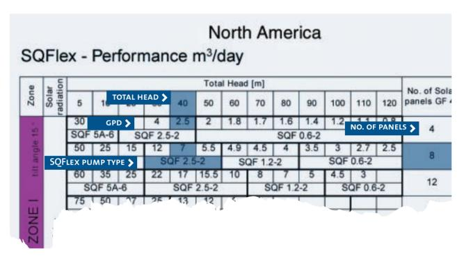
With a required total head of 40 m, and a daily water requirement of 7 m<sup>3</sup>, the correct pump is an SQFlex 2.5-2. Furthermore, the number of solar panels necessary to power this SQFlex system is 8, corresponding to 344 Wp.
