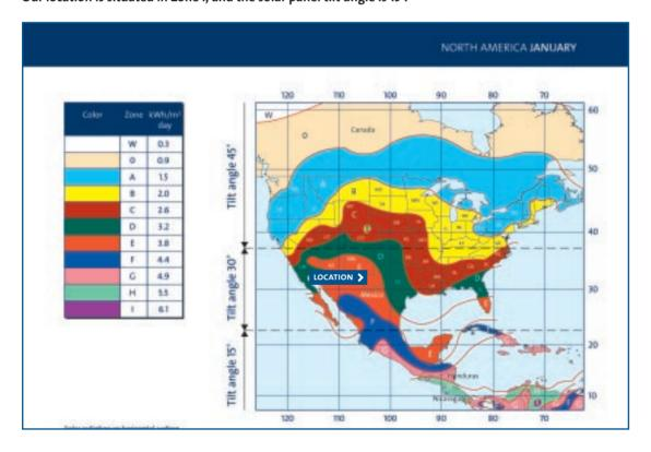
Now, it is possible to choose the relevant sizing chart according to the given zone and colour. Here's where the total head and water requirements are used to select the correct pump and number of solar panels.
