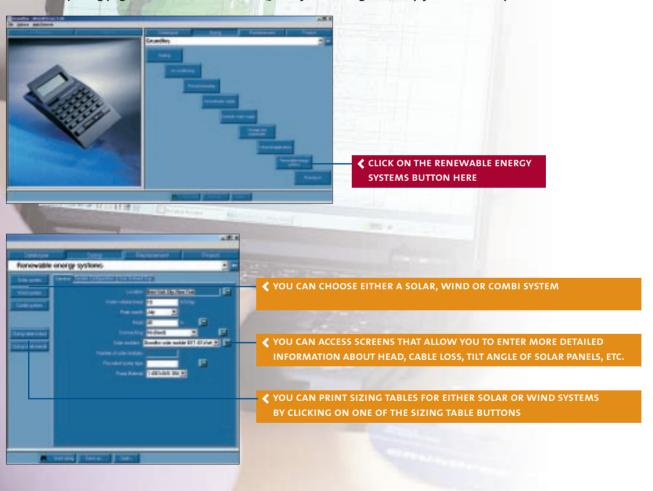
Having selected the relevant system (in this case SQFlex Solar), the program is almost ready to calculate the exact configuration. First you must enter your relevant data into the following parameters:
