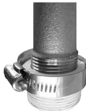
Hose clamp reinforcing a plastic reducer bushing
