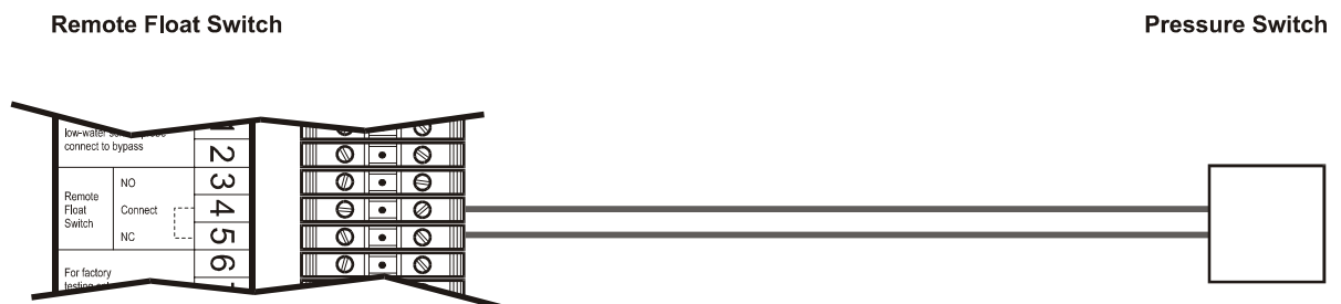
Pressure switch connected to the controller (junction box) for “remote switching”
