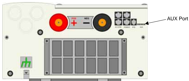
Figure 2-16 AUX Port Location
