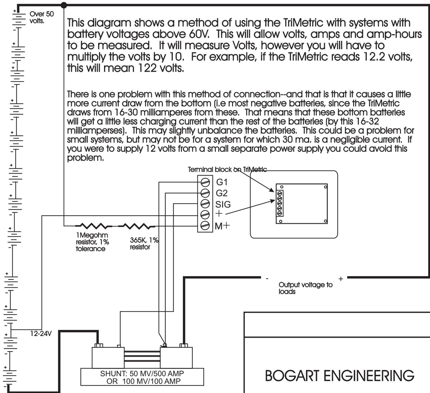
This diagram shows a method of using the TriMetric with systems with battery voltages above 60V. This will allow volts, amps and amp-hours to be measured. It will measure Volts, however you will have to multiply the volts by 10. For example, if the TriMetric reads 12.2 volts, this will mean 122 volts.
