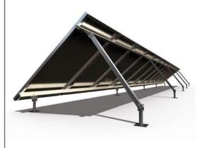
Attach IronRidge tilt legs when you need to optimize power. Our extruded legs are pre-cut to the exact length that will provide the desired angle -- up to a maximum of 50 degrees -- without requiring your installers to measure or cut on the job site.
