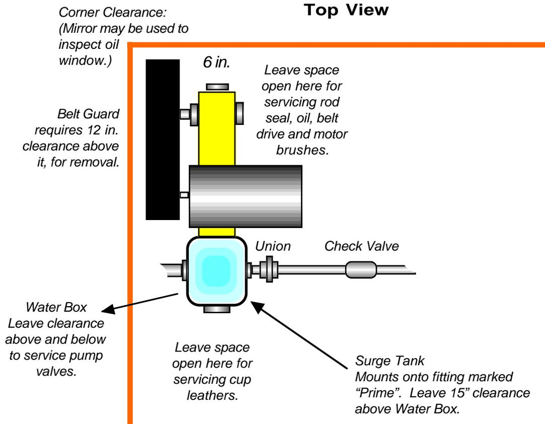
*Bolt the pump directly to a strong, firm surface. Do not mount on rubber pads.*
