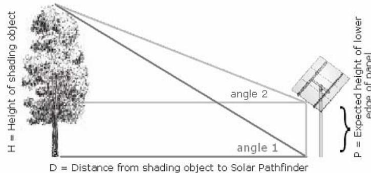
1. Place the Solar Pathfinder (SPF) on the ground in the location of the future PV panel. Using the grease pen supplied, trace around the shading objects directly onto the clear plastic angle estimator (also supplied with the SPF). The SPF clear angle estimator is write-on/wipe-off.
