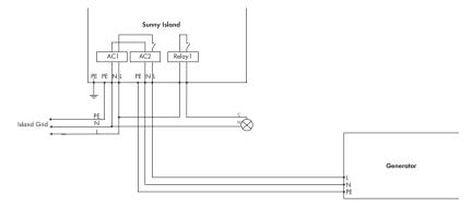
The generator is also always switched off manually. The Sunny Island 5048U then automatically switches into the operating mode without the generator.
