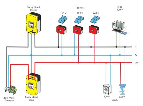
Generally speaking the relays of the slave unit will only closen when the master relay also closes.
