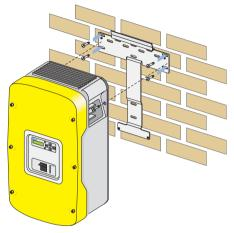
If the Sunny Island 5048U is to be installed on studs, then use the holes in the wall bracket as shown in the figure. Ensure that the wall bracket is positioned over a wall stud.Note that the wall mount bracket is designed to mount on a single stud or on 2 studs. When mounting to studs use minimum of four 5/16" lag screws with a minimum length of 2". Make sure that the wall where you intend to install the Sunny Island 5048U is vertical and can
