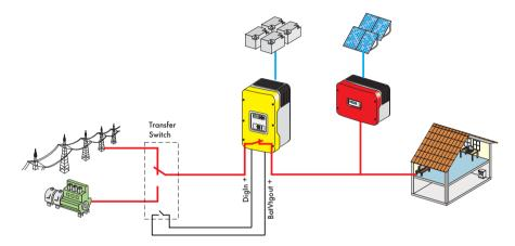
To use such a switch, do the wiring as follows:
