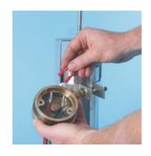
4. Place the push plate across the two motor nuts with center hole facing up.
