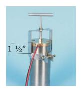
2. Hold the pump with one hand while turning the top nut clockwise, using a 9/16" wrench, until the end cap is completely out of the housing.
