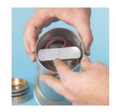
5. Reinstall puller and place the end of the threaded rod inside the center hole of the push plate.
