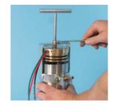
3. Remove end cap and disconnect the motor wires.
