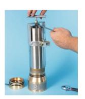
7. Remove the stainless steel housing and push plate.
