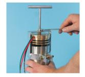
3. Remove end cap and disconnect the motor wires.
