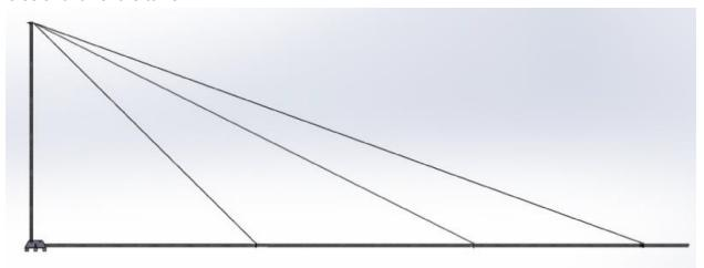
For a guyed tower there is no need for a large tower foundation, depending on the land there may be no need for a foundation at all. Two 6 foot ground rods are used at the tower base for
