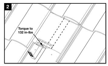
Position base over rafter, adjust arm if necessary and torque hardware to 132 in-lbs (11 ft-lbs). Position arm near center of valley for curved tiles, and away from joining seam for flat tiles.
