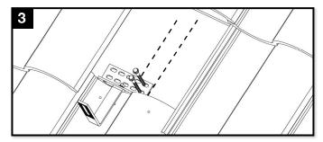
Use base as guide to drill 1/4" pilot holes, then fill with roofing manufacturer's approved sealant. Insert lag bolts and tighten until fully seated. IronRidge offers an optional aluminum deck flashing. Other approved flashing methods include user supplied adhesive backed flexible flashing.
