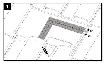
Place strips of reinforcing fabric over mastic to cover about 2" from All Tile Hook flashing edges. Sides first, then top.
