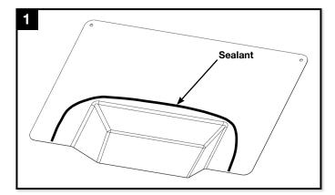
Apply a continuous line of roofing manufacturer's approved sealant on underside of the All Tile Hook flashing to form a U shape around raised edges.
