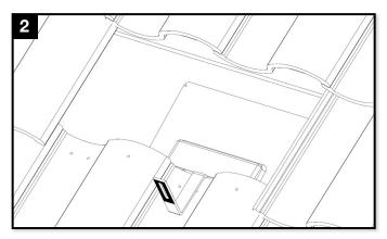
Position the flashing over the base of All Tile Hook so that the flashing completely covers the base.
