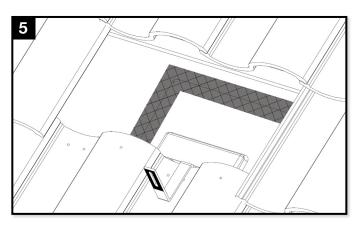
Apply another layer of mastic to completely cover the fabric. The flashing is now installed and sealed in accordance with TRI Guidelines.
