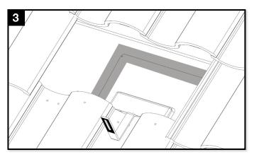
Begin three-course sealing method by applying a layer of mastic over edges of All Tile Hook flashing. Felt paper bibbing over flashing is also acceptable.
