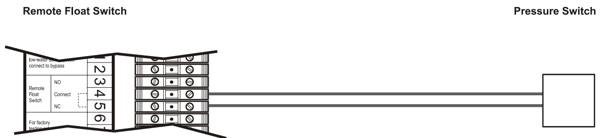
Pressure switch connected to the controller (junction box) for "remote switching"
