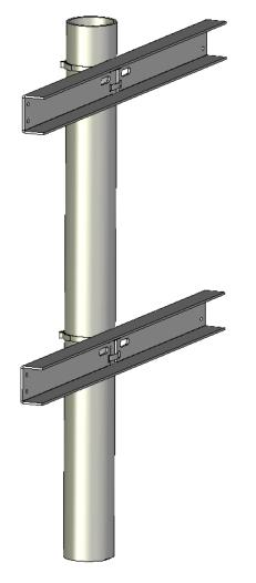
3. Once the hose clamps are in the desired position, tighten the hose clamp screws to 35 inch-lbs.
