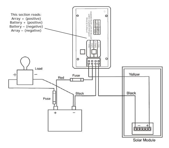
It is advisable to install an inline fuse on the positive connection of any wire connected to the battery. The fuse should be within 12" of the battery.
