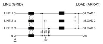
Connect both the Enphase Envoy and Enphase Microinverters on the array or load side of the filter, and wire the utility feed to the line side of the filter.
