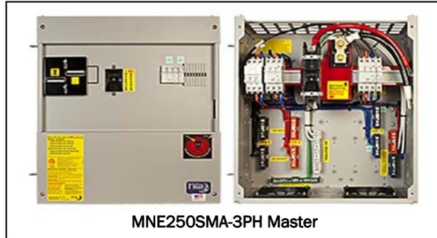
The three phase master includes the three phase 60amp input/output bypass system. This E-Panel can be used in conjunction with a Sunny Island inverter as part of a three phase off-grid, battery backup or AC Coupled system. Terminals are provided for hookup to leg two and leg three E-Panels. Comes with 250amp battery disconnect breaker and inverter cables. This unit is pre-wired with AC input and output wiring for leg one (master) inverter. (Two slaves are also required for three phase.)
