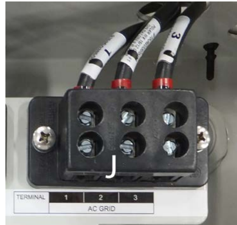
Figure 3-18: Bottom switch AC grid terminal
