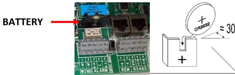
Figure 6- 1: Internal battery replacement
