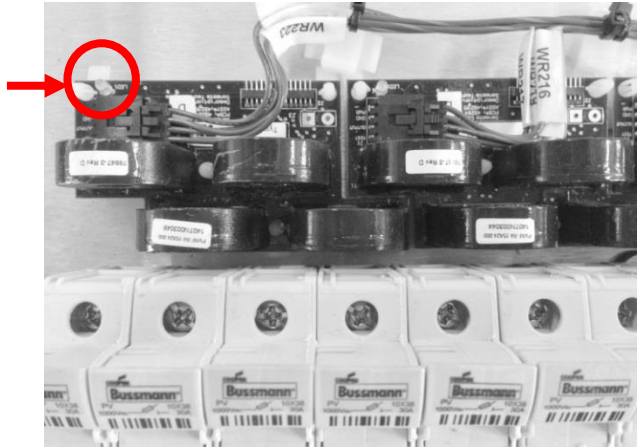
Picture 6 – Arc Sensing Boards and LED Indicators
