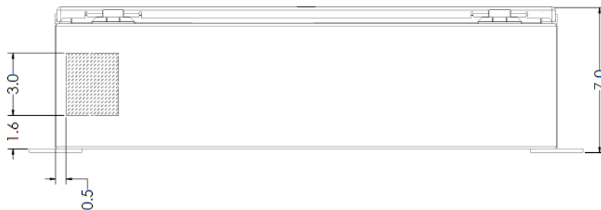
Figure 3 – Conduit Entry Locations, Left Side (Based on vertical mounting)
