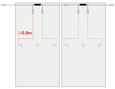
NOTE: The output cable length of integrated junction box PV module should be no less than 0.9m.
