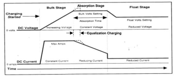
(Lead-Acid Battery Three-Stage Charger)
