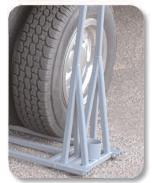
Position the base support frame ahead of the tire.
