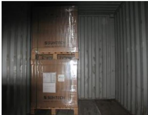
The width of a carton box is nearly half of the width of a 40 foot high cubic container, which enables two lines of carton boxes to be packed in a container, and prevents possible inclination of carton box during shipment.
