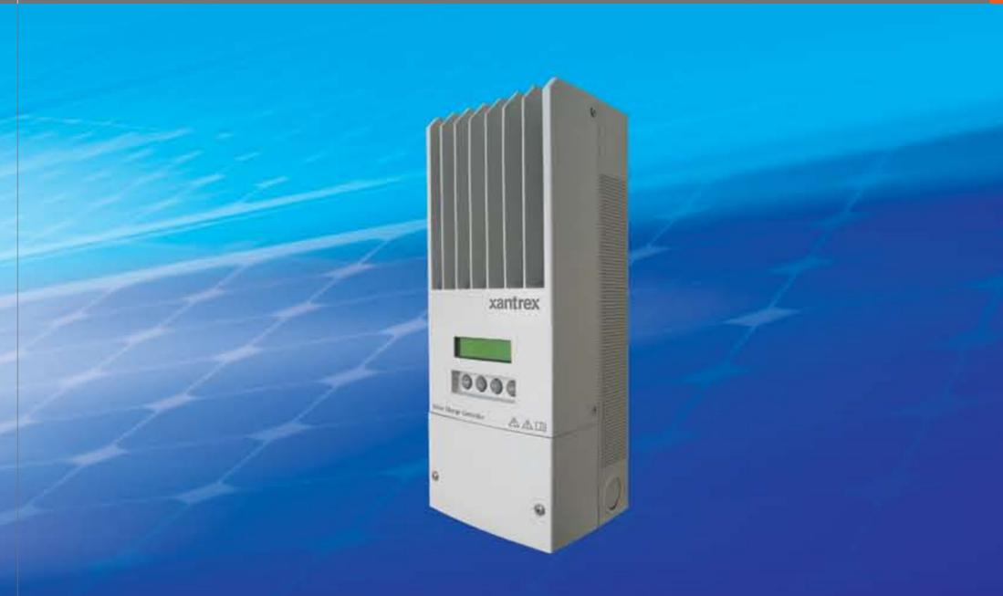
The Xantrex Solar Charge Controller (XW SCC) is a photovoltaic (PV) charge controller that tracks the electrical maximum power point of a PV array to deliver the maximum available current for charging batteries. The SCC can be used with 12, 24, 36, 48, and 60-volt DC battery systems. The Solar Charge Controller is designed to regulate PV input only. It is not designed to work with wind or hydro generators.
