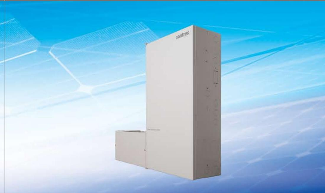
The XW Power Distribution Panel (XW PDP) with conduit box is factory-wired and labeled to support a code-compliant single-inverter installation. It is factory configured to mount on the right side of the inverter/charger and may also be mounted on the left side. Internal wiring and breakers can be added to expand the XW System with up to three inverters, four charge controllers, or other equipment to support larger systems.
