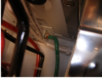
Chassis ground connection to inverter
