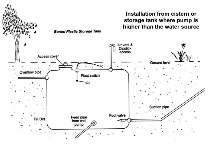
NOTE: It is preferable to place the pump LOWER than the water level in the tank. This illustrates an alternative, not an ideal. Note the upward rise of the suction pipe, the high position of the priming plug, and the horizontal position of the filter. These measures help prevent air entrapment that restricts flow and causes pump noise.
