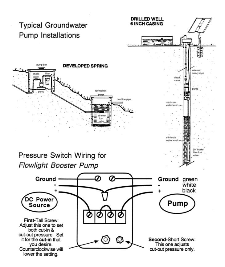
**Explanation:** The National Electrical Code® specifies that switches <u>not</u> disconnect the "grounded conductor", which is the negative. So, we are switching only the positive. Using both sets of contacts as shown (in series) will extinguish the arc (spark) that forms when the contacts break. This greatly increases switch reliability.
