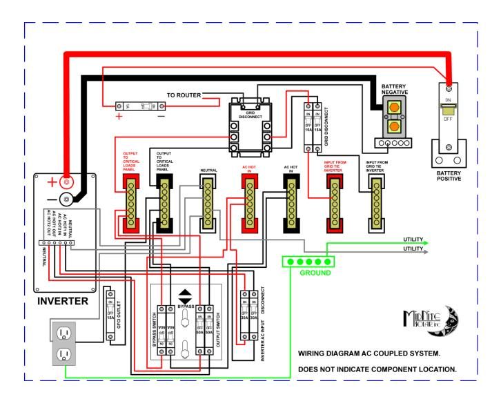
Before starting this project please make sure the Grid tie inverter is off line and make sure you follow all necessary safety precautions. Always shut off all AC power before working on any circuits. Also make sure to switch off the Battery breaker in the AC coupled system before installing batteries.
