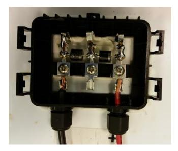
Solder wires onto attached terminals.
