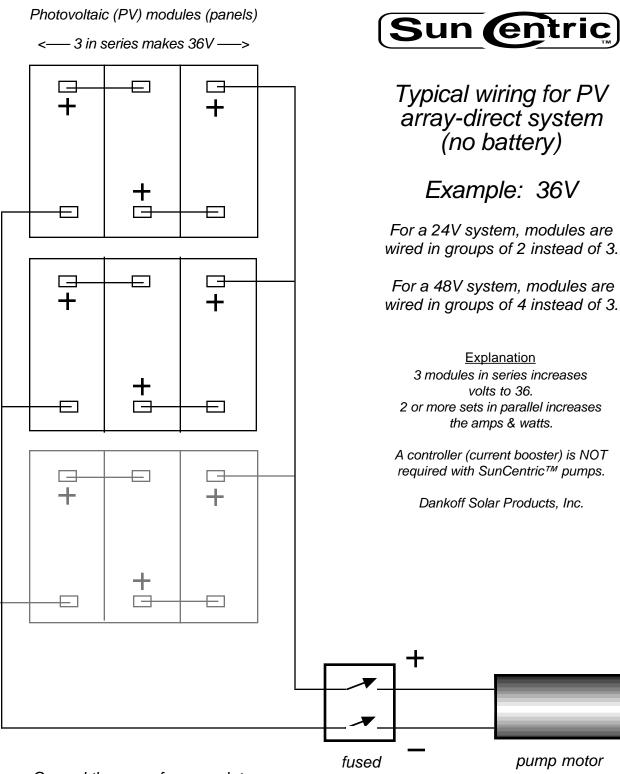
Ground the array framework to earth for lightning protection. Do NOT ground the power negative. disconnect switch
