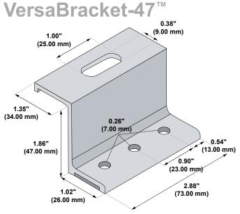
3 holes are provided for versatility. Some installations require only 2 fasteners. See the load table on the S-5! website and the installation instructions for more details.
