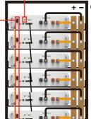
(3) Wait a few seconds and the batteries will automatical turn on one by one, until all the running lights flash,indicating that the batteries are working properly.
