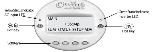
Six buttons or keys navigate the MATE and change its settings:
