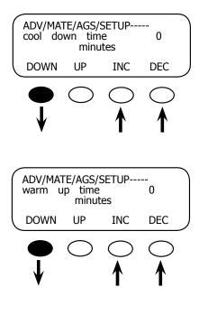
After the FX charging has been disabled, the *cool down time* screen allows the user to adjust the number of minutes the generator will cool down before being shut off. This time should follow the manufacturer's recommendations. Press the **<DOWN>** key to view the warm up time screen
