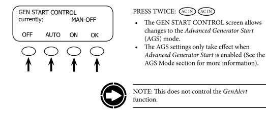
• When an OutBack HUB is employed, the GEN START CONTROL only affects the FX programmed as the AGS PORT in the AGS setup. This is the HUB Port connected to the FX with the generator start relay.
