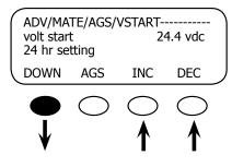
If the battery voltage falls below this set point, a 24 hour timer starts counting down. Upon reaching zero, a start command is sent to the generator unless it is currently Quiet Time. To change the default settings, use the **<INC>** and **<DEC>** soft keys. When finished, press the **<DOWN>** soft key to go to the *volt start 2 hr setting* screen.
