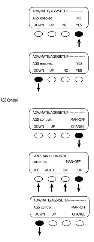
This is the overall control for the AGS Mode. If AGS is not enabled, none of the AGS settings or controls will work. Enable the AGS first by pressing the **<YES**? soft key and then establish your settings.
