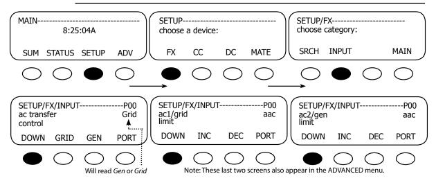
Grid-Use Mode allows programing the times the FX system connects to an AC input source and enables the **USE** mode. The time and date must be accurately programmed for Grid-Use mode to function properly.
