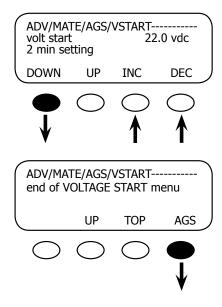
If the battery voltage falls below this set point, a 2-minute timer starts to count down. Upon reaching zero, a start command is sent to the generator even if it is currently Quiet Time. Use the **<INC>** and **<DEC>** soft keys to change the default settings. When finished, press the **<DOWN>** soft key to go to the *end of VOLTAGE START* menu.
