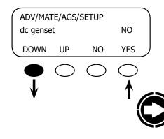
In this screen, YES means a DC generator is present and the AGS routine, which normally stops the generator upon the FX going to Float or Silent, will instead stop the generator when the *vdc genstop* setting is reached.
