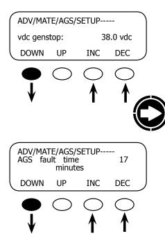
This voltage setting will terminate a Voltage Start command when the battery voltage remains above it for 15 minutes regardless of the DC Genset setting. The setting can be adjusted using the <**INC**> and **<DEC**> soft keys. Press the **<DOWN**> soft key to view the AGS fault time screen.
