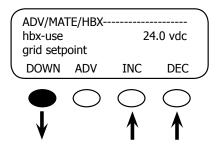
This is the voltage set point that allows the FX to connect to (USE) AC power. The battery voltage must remain below the voltage listed on the screen—24.0 vdc in this case—for the amount of time programmed by the HBX-USE GRID DELAY (see next screen) before a USE command is issued. Use the **<INC>** and **<DEC>** soft keys to change the voltage set point. Press the **<DOWN>** soft key to proceed to the next screen.
