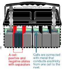
oxide on the plates and sulfuric acid in the electrolyte, for the most part.
