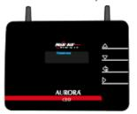
Choose the installation location of the CDD to configure the WiFi network and acquire the Micro Inverter. It is advisable NOT to fix the CDD to the wall in order to evaluate the placement based on the signal range.
