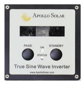
Figure 1.0: TSW Control Panel
