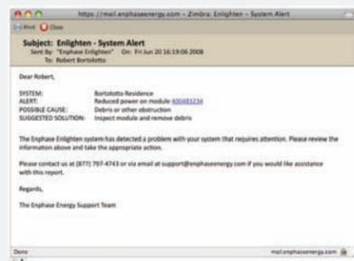
Enlighten promptly sends an alert to the system owner or installer per the user-defined preferences established at installation.
