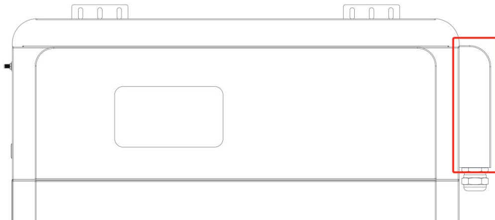
Figure 3.6.1. Removal position of the battery control module
