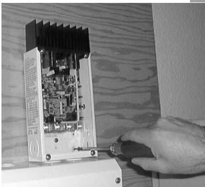
Figure 2-3 Mounting the C-Series Multifunction DC Controller
